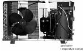
Figure 38: Pool water temperature sensor.
